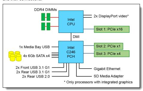
Figure 5. ST50 system architectural block diagram
